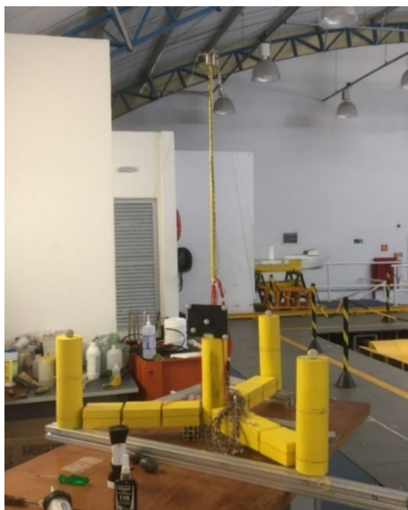
Fig. 3 Elastically and dynamically similar segmented backbone model
