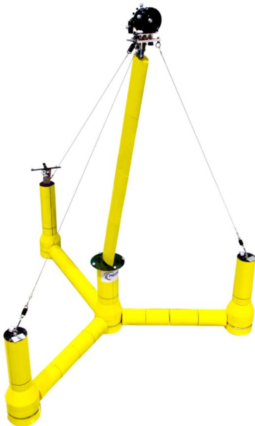
FIGURE 2 ELASTIC AND DYNAMIC SIMILAR SEGMENTED BACKBONE MODEL USED IN THE EXPERIMENTS
